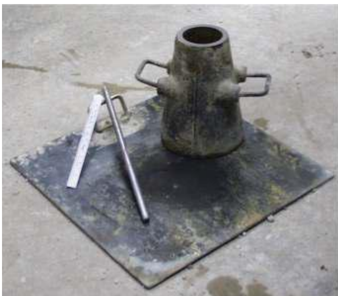
Appendix 8: Picture of a slump cone.
