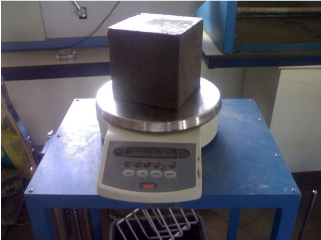
Appendix 7: Picture of a concrete cube being weighed
